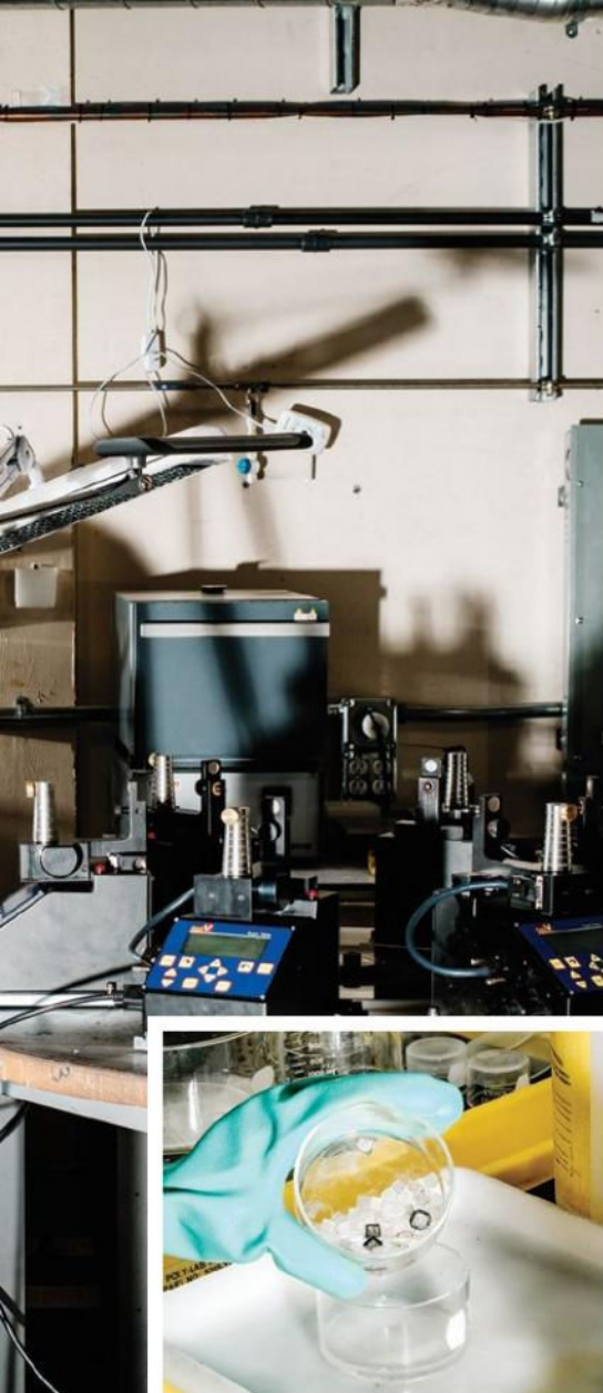
New diamonds come out of the reactor covered in a dark film of carbon. Jeremy Scholz, Diamond Foundry's CTO, cleans them to prepare for cutting and polishing.
