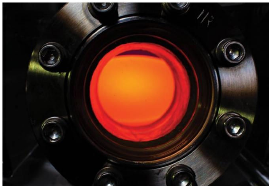
Left: Operational from 1871 to 1914, the Kimberley diamond mine in South Africa, called the Big Hole, was dug entirely by hand with picks and shovels. Below: A look inside Diamond Foundry's plasma reactor, in which 8,000-degree plasma deposits new layers of carbon onto a "seed" diamond.
